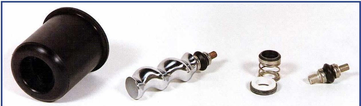
The key to the EP's performance is its simplicity. The only moving part is a helical screw rotor that turns inside a rubber stator, creating a tightly sealed cavity that progresses from the suction port to the discharge port. This proven design utilizes positive displacement to deliver uniform, continuous flow of almost any liquid. The end result is lower maintenance requirements, economical operating costs and solid reliability.
